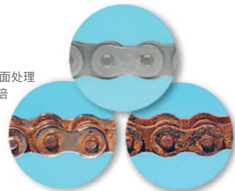
After 60 days of outdoor exposure Hydro-Service® demonstrates the rust resistance that makes it the best choice for outdoor use. 60天暴露在外，Hydro-Service® 显示出防锈性使他成为室外应用的更佳选择。
