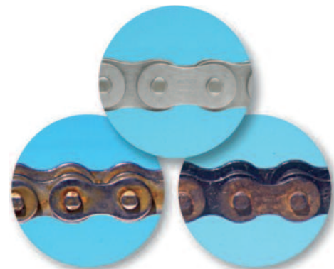
After 14 days in and out of a 5% saltwater solution (equivalent to sea water) it can be seen that the Hydro-Service® coating will extend the chain life compared to onventional nickel plating or carbon steel in more challenging applications. 14天在5%盐水（与海水相近）中浸入和浸出，可以看到在更具有挑战的应用中Hydro-Service® 镀层与其他传统镀镍链板或碳钢相比更可以延长链条寿命。
