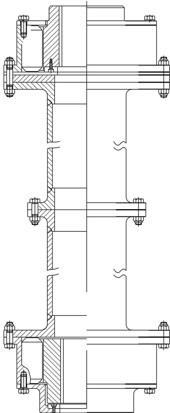
Spacer Couplings. Used to increase the distance between shaft ends and allow access to driven and driving machine.
