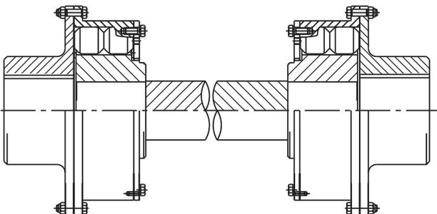
Cardan Shaft Coupling. Used to increase the distance between shaft ends and give a higher misalignment capability.
