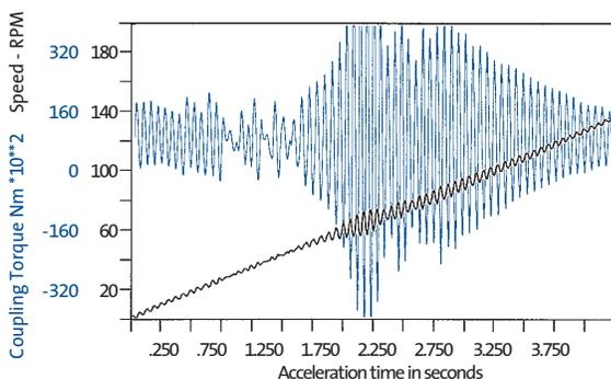
Table C shows a typical motor/fan system connected rigidly (or through a gear or membrane coupling) when damaging torques would have been experienced in the motor shaft.
