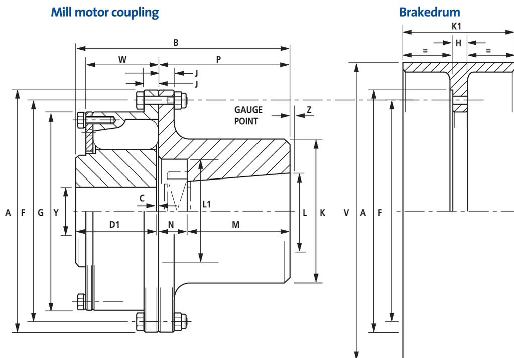
Brakedrums may be used in conjunction with the whole range of PM couplings and may be bolted on either the driving flange or flexible half side of the coupling, the recess -  $\phi A$  - locating on the outside diameter of the coupling.
