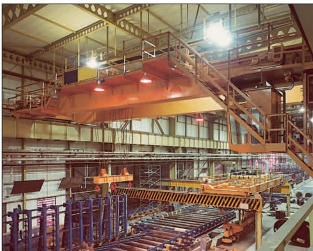
Steel mills. Couplings fitted on 35 ton overhead crane, and on table roller drives.
