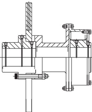
Combination with a brake disc, for use on cranes, fans and conveyor drives. (Brake drum couplings also available).
