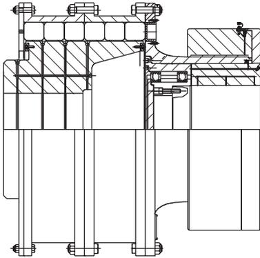
Combination with a torque limiting device to prevent damage to driving and driven machine under shock load.
