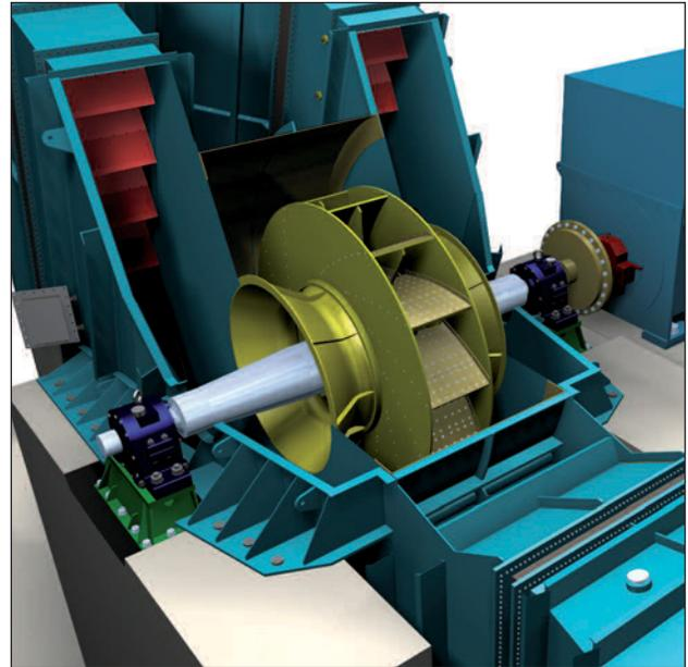
Fan Drive. Coupling fitted between the variable frequency electric motor and the fan.
