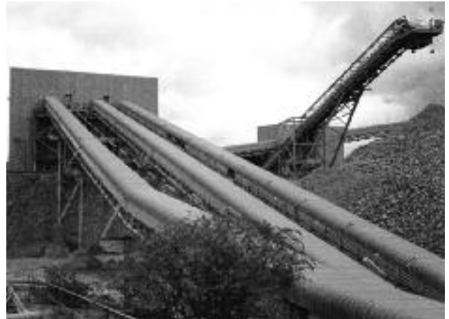
Sprag Clutch holdbacks are often used on inclined conveyor headshaft drives to prevent runback in the event of a power failure.
