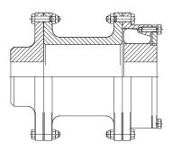
Spacer Coupling. Used to increase distance between shaft ends and allow easy access to driven and driving machines.
