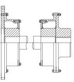
Cardan Shaft Coupling. Used to increase the distance between shaft ends and give a higher misalignment capability.
