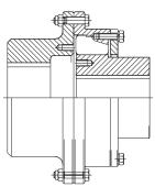
Coupling with long boss inner member and large boss driving flange to increase shaft engagement and to accept larger shafts.
